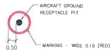
AIRCRAFT GROUND RECEPTACLE PIT MARKING
