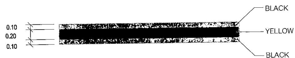
STAND LEAD-IN LINE , TAXIWAY AND TAXILANE CENTERLINE
